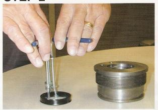
With the two handles in this position, place the center leg on the outer part of the seal with the outer legs on the inside.
