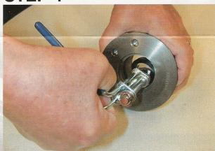
Place the seal in the groove - release and remove the tool.
