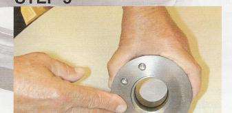
Finish by pushing the seal in the groove with your finger.
