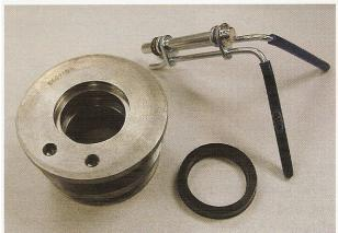
Rod u-seals usually small in diameter, are difficult to install in gland grooves. Hercules installation tools, shown on page 13 of our 2003 Master Seal Catalog simplifies this task. The following pictures show the use of the tool with a 1-3/4 I.D. rod u-seal.
